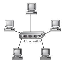
As a general rule, switches are superior to hubs. Hubs mirror all traffic to all computers, whereas switches are smart enough to send packets only to the intended destination. Switches also allow *full-duplex* transmission, in which both parties can send data at the
