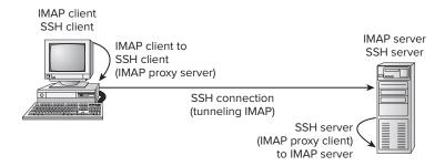
Of course, all of this requires special configuration. The default configuration on the server enables tunneling; but to be sure, check the /etc/ssh/sshd\_config file on the server for the following option:
